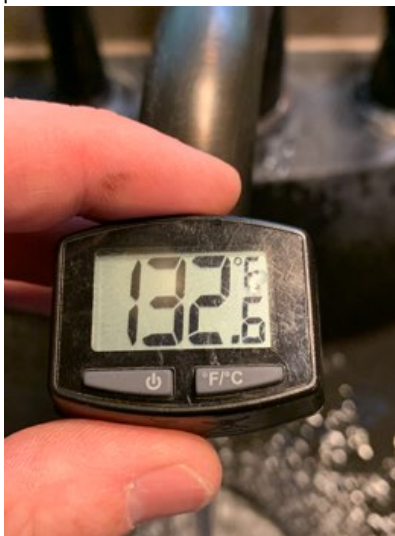
Hot water temp taken at the kitchen sink
